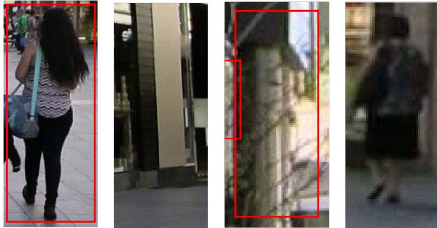
Figure 3.4: Four different results, from left two right: true positive, true negative, false positive, false negative
