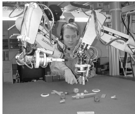
Fig. 2. Two-arm multisensor robot system for dialogue-guided assembly.
