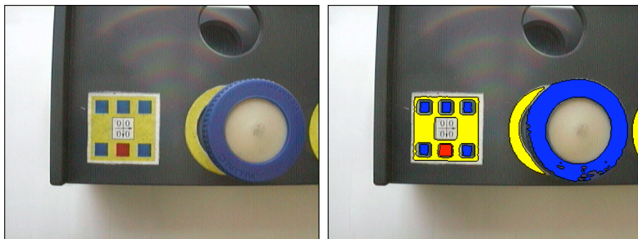
Figure 4. Image processing for object recognition. On the left the captured image of an optical marker and a 50ml tube, on the right the processed image showing the different segments for the search colours.
