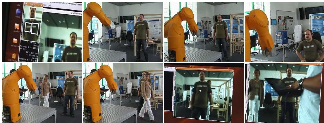
Fig. 7. Sequence with the robot controller in action. Top left: model acquisition. The sequence shows the system successfully handling mutual occlusions in a cluttered environment.
