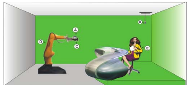
Fig. 2. Proposed model of the VR-TV studio with camera operated by a vision-assisted robot arm: A) Frontal Firewire camera for 2D person localization and tracking, B) Overhead camera for computing the moderator distance from the robot C) Broadcasting TV camera, D) Robot manipulator, E) Moderator
