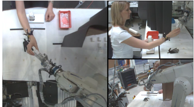
Fig. 1. Assisted assembly set-up used in the experiments. Human and robot are sitting opposite to each other on a table. Behind the black barrier invisible to the human, the robot simulates additional tasks when no assistance is needed. When the human hand crosses the black line, the robot is triggered (strategy (III)). A marker-based tracking system ( ARTrack ) is used to estimate the hand position of the human
