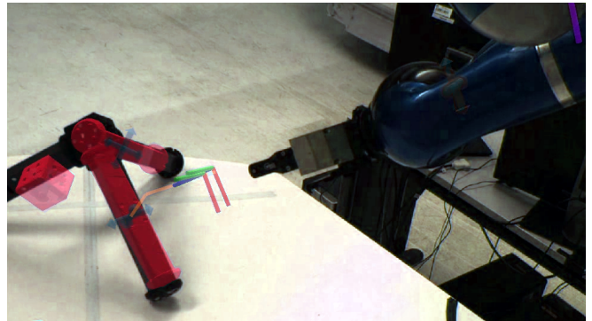
Fig. 2: A screen capture of a representative view of the operator visualization in the prototype system over a low-performance network during a sensor-based control augmentation. The GRASP-Beams (left) have been recognized by the 3D perception system and the commanded trajectory of the DLR Lightweight Robot (right) has been interpreted to dispatch a trajectory to grasp one of the parts (center).
