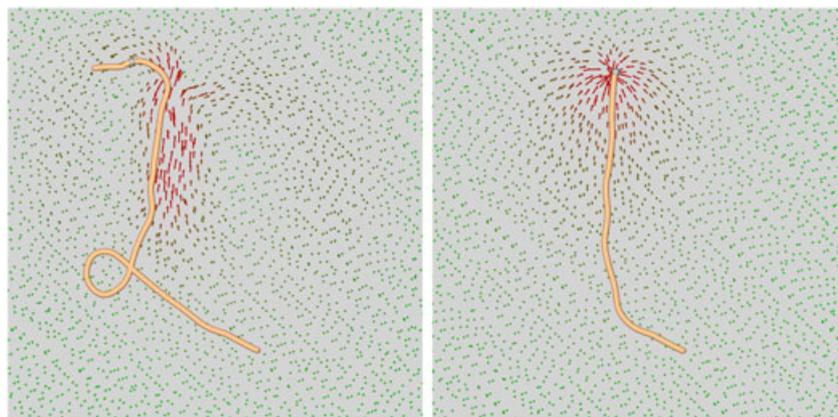
**Figure 14.** Different results of the fluid simulation for instantiation of the same tasklet when the speed of the particles are changed. Left: trajectory with particles travelling too fast, right: trajectory after speed adjustment
