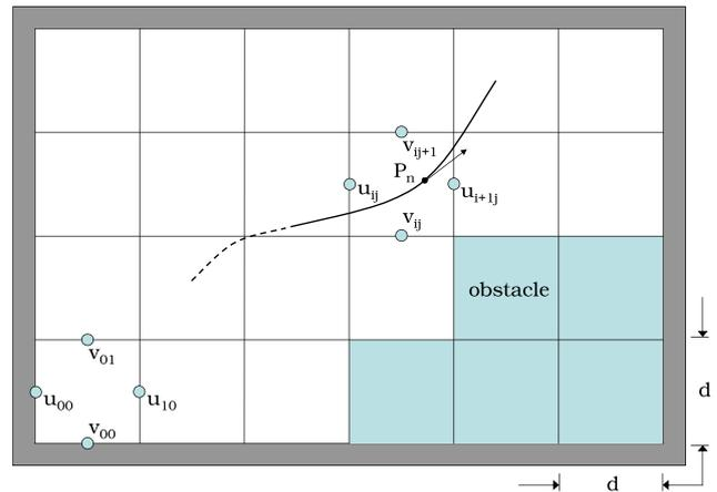
**Figure 11. Fluid simulation:** the area of interest is discretized into equally sized cells. For clarity reasons, only a limited number of cells that would be too coarse for practical use is shown in this picture – our practical implementation usually works on a grid of at least  $50 \times 50$  cells. Evaluation of velocities is not centred within a cell but distributed on a staggered grid to assert numeric stability
