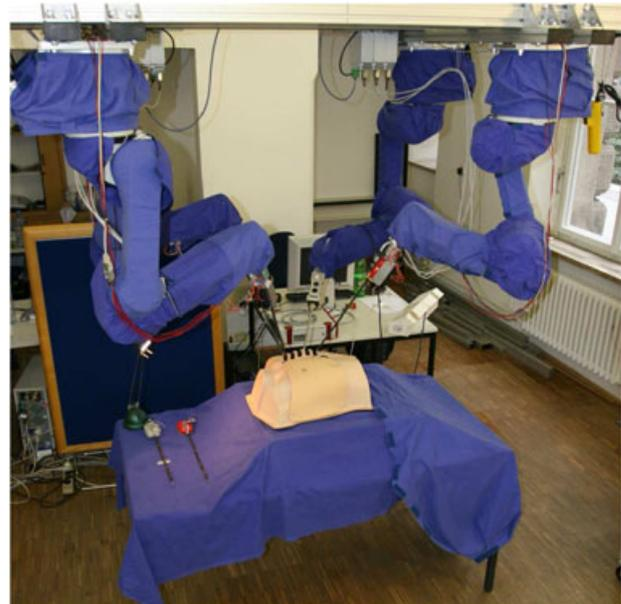
**Figure 2. Hardware setup:** four ceiling-mounted robots with surgical instruments, either a stereoscopic endoscope or different surgical microgrippers. The minimally invasive instruments are augmented with force sensors. In-output is accomplished at a master console, comprising two force feedback devices
