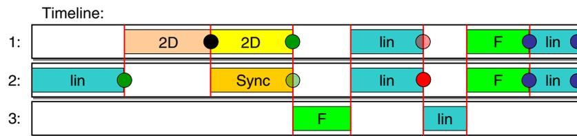
Figure 9. Knot-tying task as a sequence of tasklets. (lin, linear motion, 2D, two-dimensional primitive, F, force primitive)
