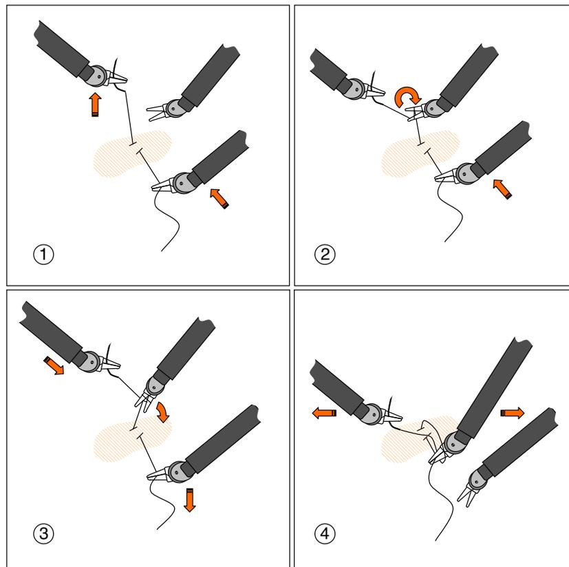
Figure 3. Automatic tying of a knot: four phases of an automatic tying procedure performed with three instruments
