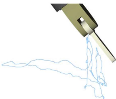
Figure 5. *Knot-tying trajectory*: visualization of a typical recorded trajectory of the left gripper during knot-tying, as commanded by a human surgeon
