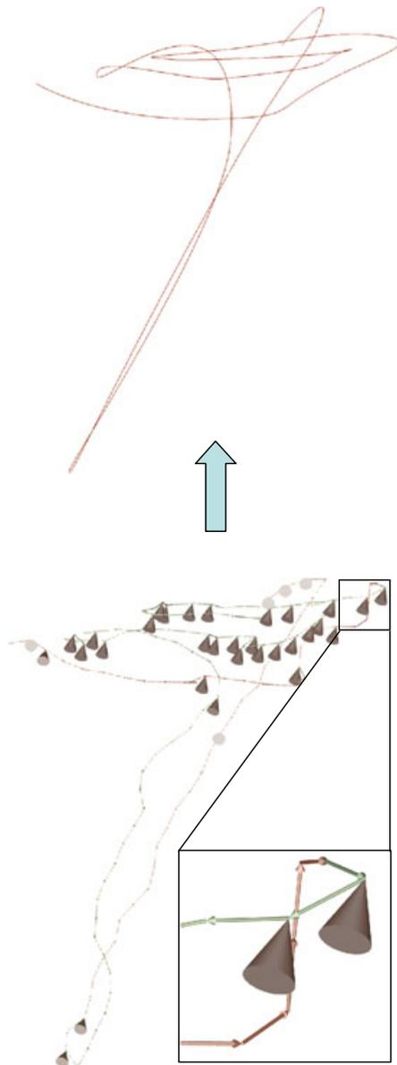
**Figure 6. Spline approximation:** Significant events are selected from the recorded trajectory (cones on left image). These points serve as breakpoints for a spline approximation of the trajectory (right image). Note that human tremor is suppressed, while all significant edges are preserved
