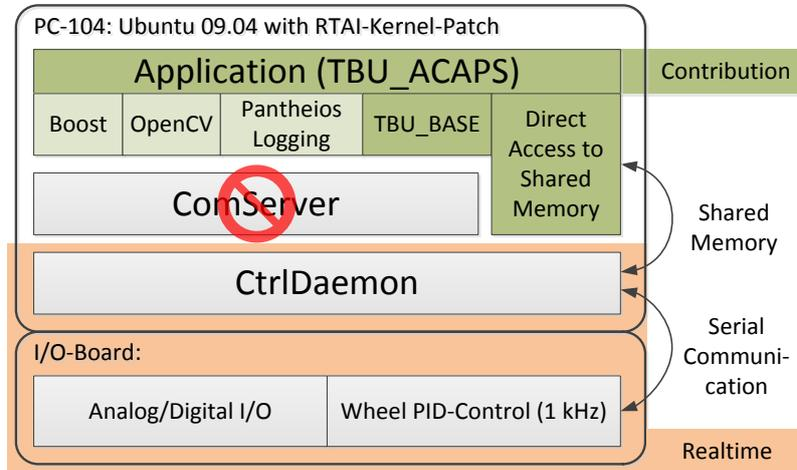
Fig. 3: Overall Robotino software layers with our software code on top of the realtime components of the standardized Robotino platform.
