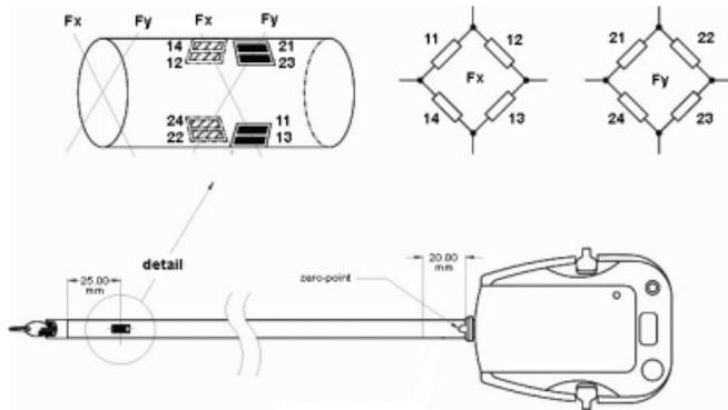
**Figure 2** Application of strain gauge sensors. One full bridge for each direction in X and Y.
